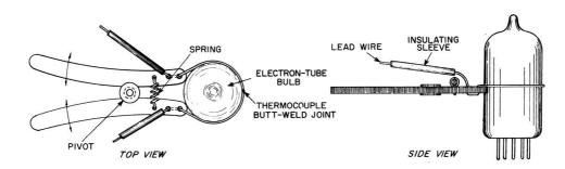
The loop is placed about the bulb and adjusted so that the thermocouple junction coincides exactly with the bulb hot spot, which has been located by the Tempilaq technique. The loop is then clamped tightly against the bulb surface, and the temperature is read on a chromel-alumel potentiometer indicator. This method has demonstrated excellent repeatability, and is especially useful for determining plate dissipation.
